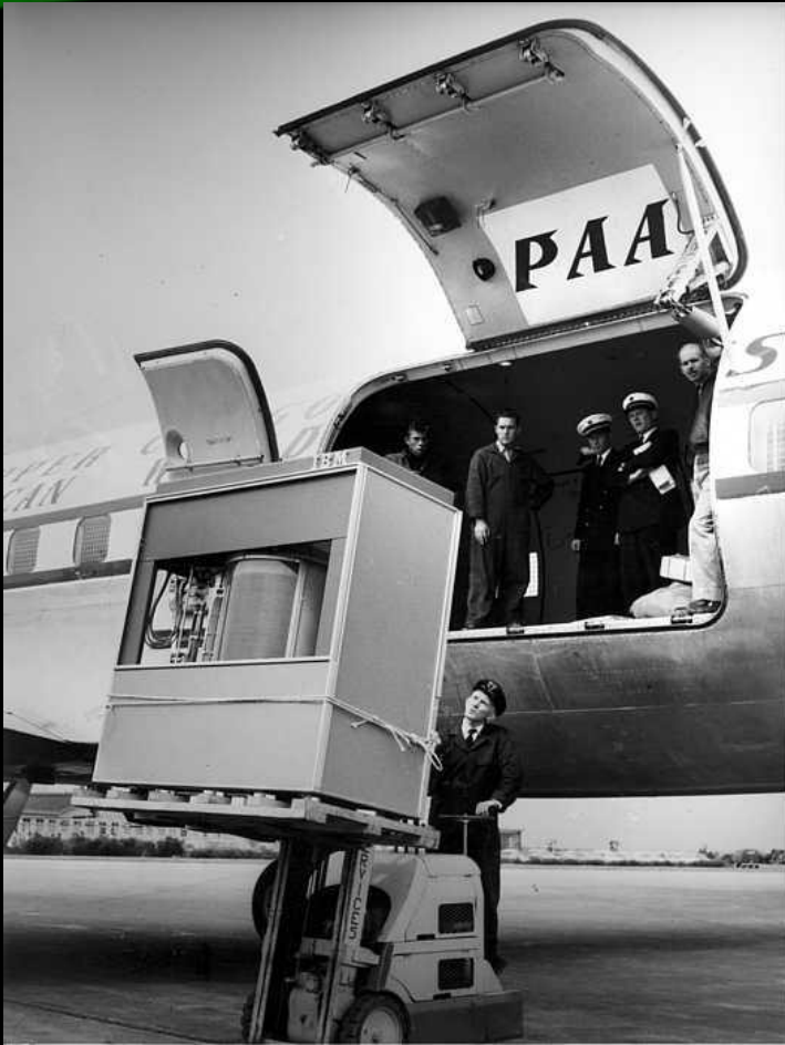
1956: World's first hard disk: IBM 350 weighed over a ton. Oh, it was 5 MB.
